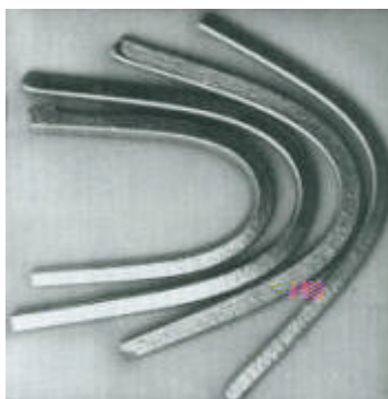
Brittle alloy bars bent in Hasted's experiment
